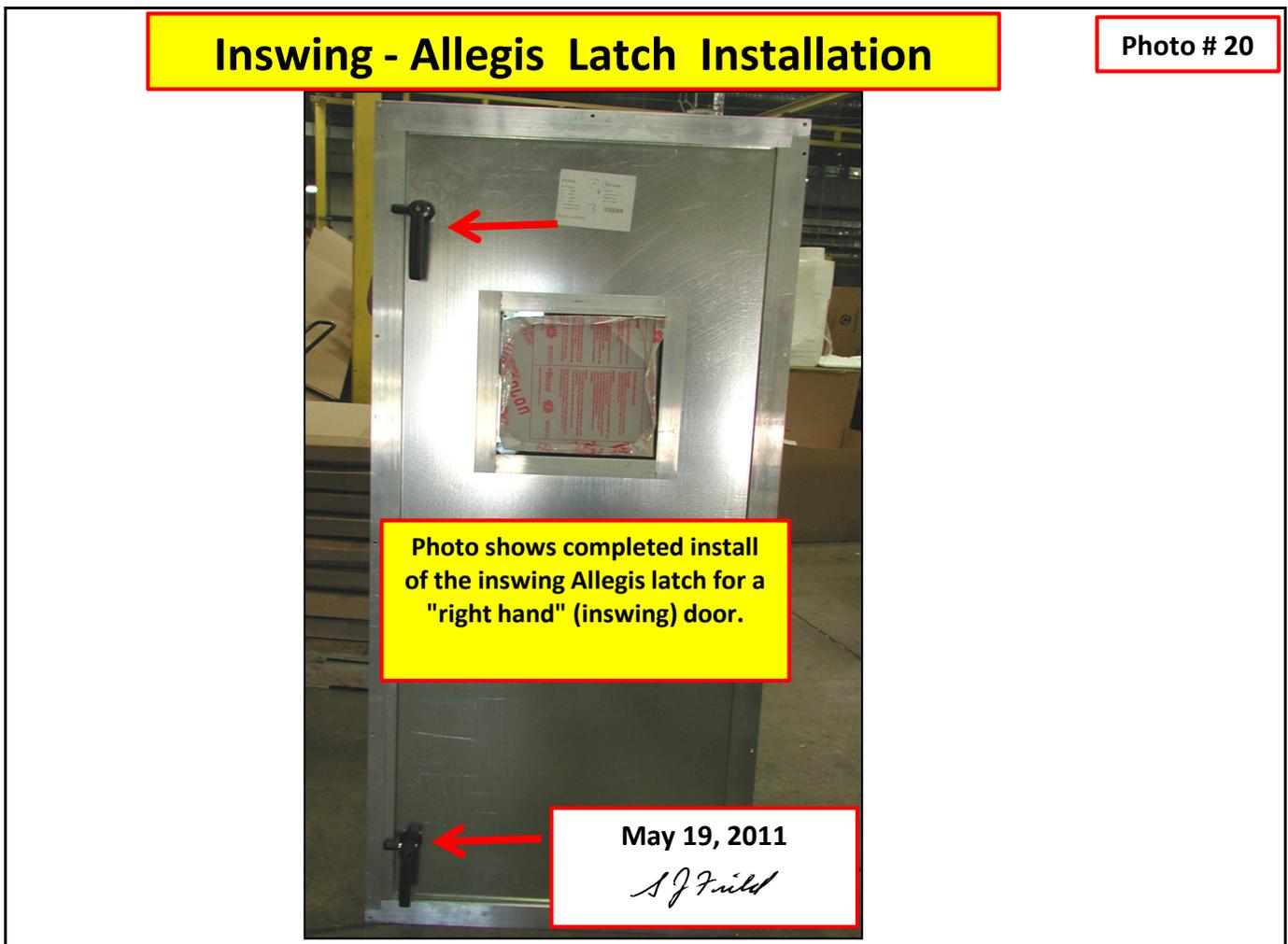
Photo shows completed install of the inswing Allegis latch for a "right hand" (inswing) door.
