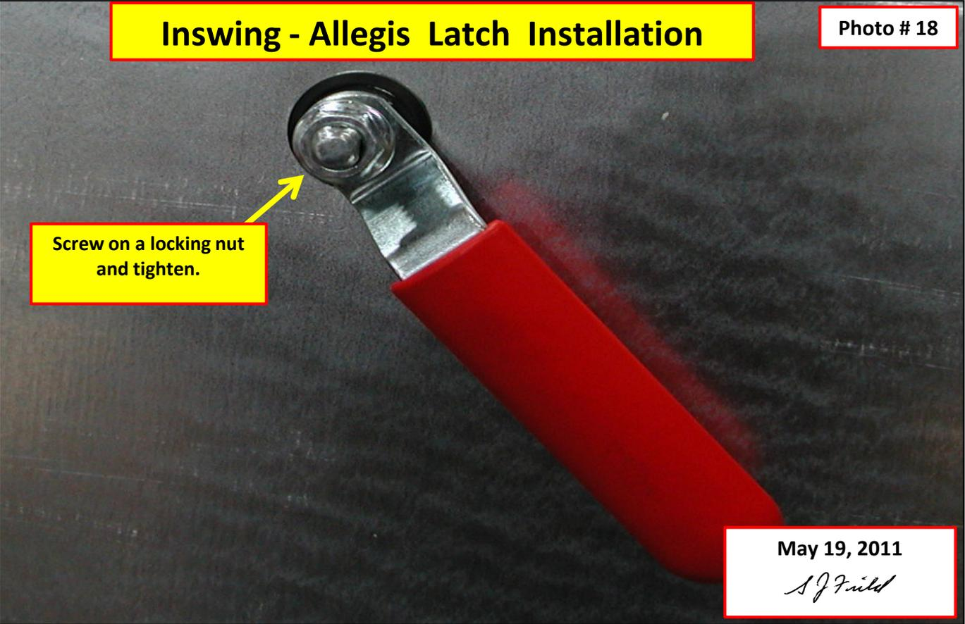
Screw on a locking nut and tighten.
