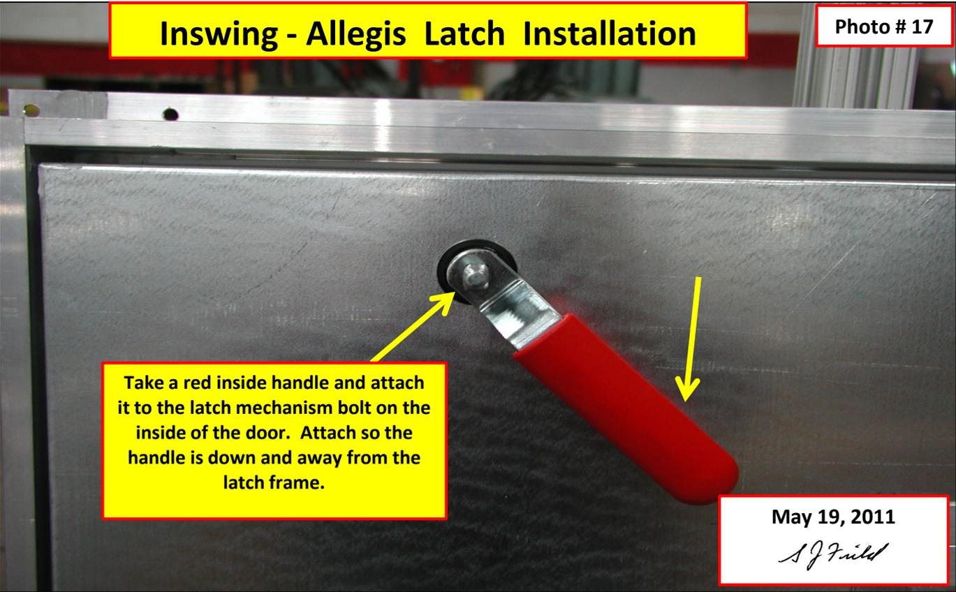
Take a red inside handle and attach it to the latch mechanism bolt on the inside of the door. Attach so the handle is down and away from the latch frame.
