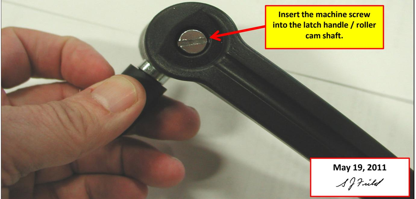
Insert the machine screw
