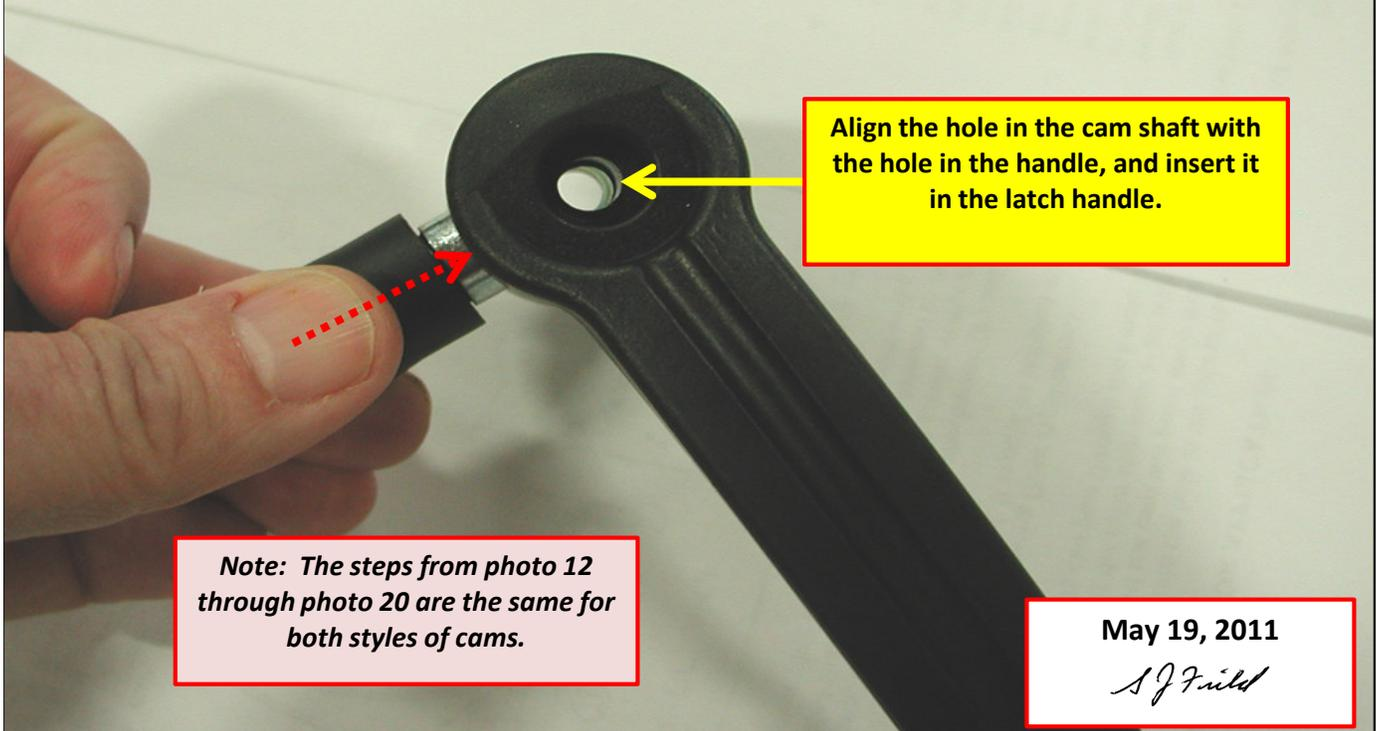
Align the hole in the cam shaft with the hole in the handle, and insert it in the latch handle.
