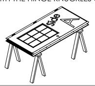
AFTER REMOVING THE THE RETAINING CLIP AND FRAME SPACERS, OPEN THE DOOR.
