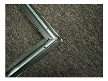
**NOTICE:** Please note that both the "inside" and "outside" portions of the view port have "This End Up" stickers on them. When doing step 3 below, to insure alignment of the screw holes in the two halves of the frame, be certain that the frame sections are oriented so that the stickers are positioned the same on both sides of the door panel.
