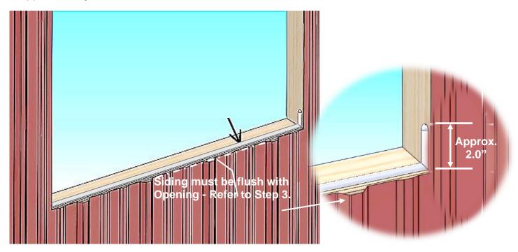
8. Apply sealant to the siding face on both Vertical sides, starting just below the top corner slots, with a 3/8" –1/2" bead extending down slightly past the sill. Also apply a dab of sealant between the siding and wood at the bottom two Sill corners.
