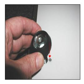
3. On the interior side of the panel, place the provided Escutcheon w/ Tinnerman clip onto the Latch Mechanism shaft with the smaller diameter collar side towards the panel. Push the escutcheon all the way down the shaft and into the pre drilled latch hole.
