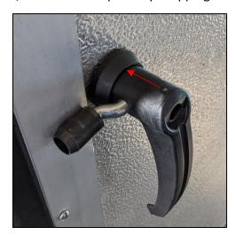
9. Apply the release handle, positioned away from the latch frame, to the Latch Mechanism shaft. Apply the locking nut and tighten down. Operate handles for verification of proper installment.
